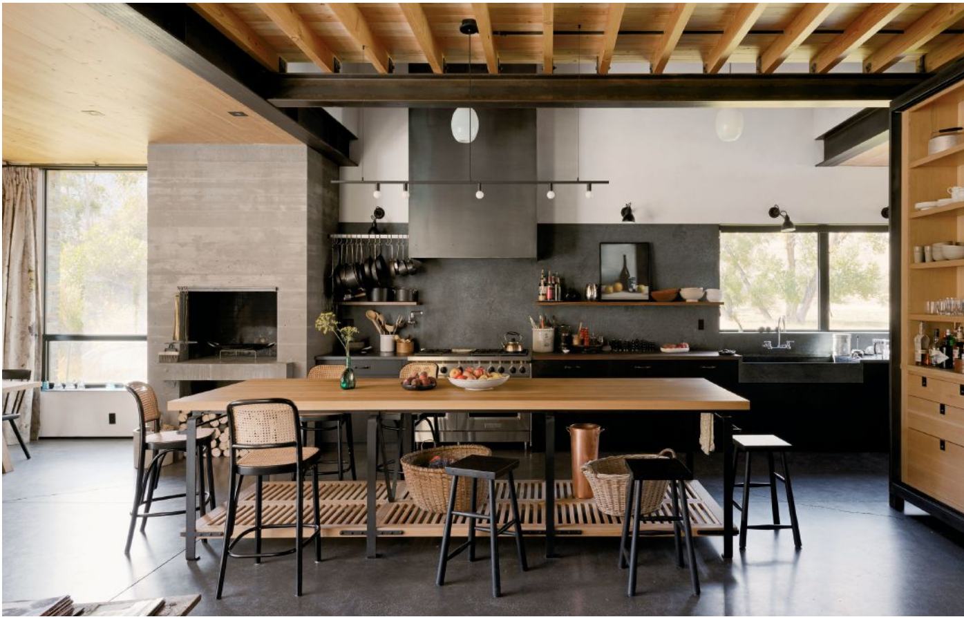
This page: The open kitchen reveals the sturdy structure of the house, fortified by steel for seismic loads. Faced in board-formed concrete, an Argentinian wood-fired grill anchors one end of the cooking wall. Soapstone counters top the ebonized wood cabinets, and Douglas fir paneling clads the ceilings. Concrete floors are geothermal radiant.
